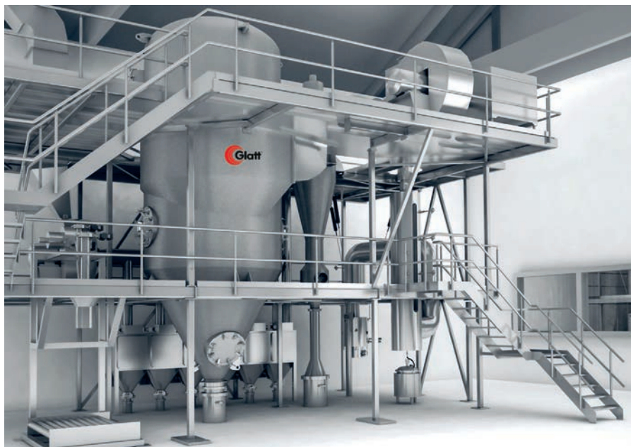
Fig. 6 ProAPP® 500 plant for the production of high-performance powders (Source: Glatt Ingenieurtechnik)
