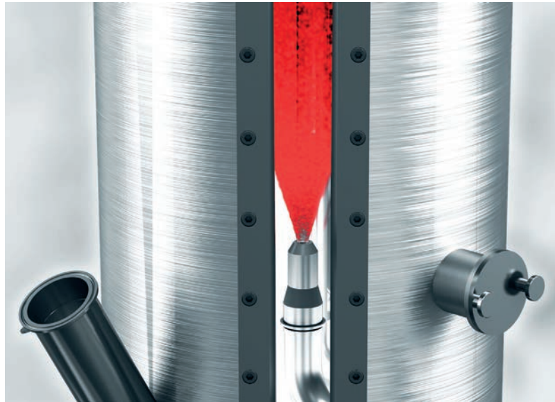
Fig. 2 In the synthesis reactor, only the gas flow pulsates in a controlled manner in the specially designed reaction chamber; for particle production, fine droplets of a raw material solution are sprayed into the gas stream to form particles
