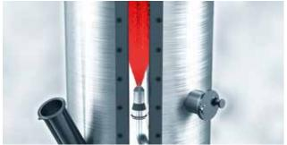
Precursors are sprayed into the pulse gas stream
